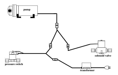
TSO: full tank shut-off switch, pressure switch ESO: electronic shut-off valve, solenoid valve
